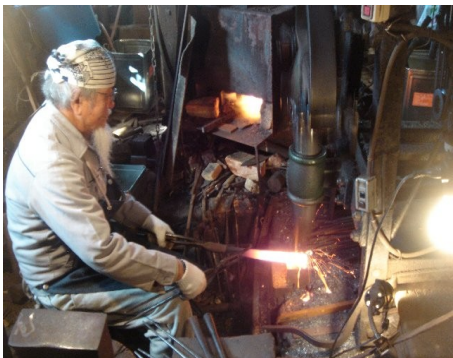
Smiting around 1,200degrees and removing the rust of surface. Making rectangle section.
