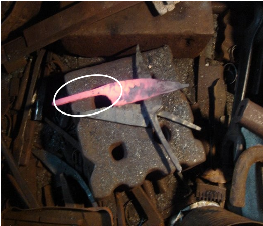
Stretching the core
