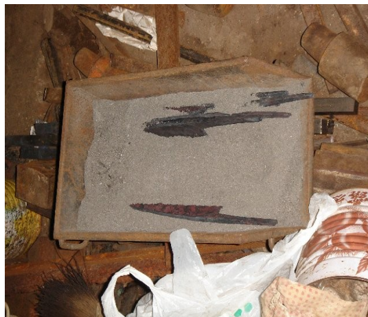
After Hosakinobe ,it's Annealing process. Putting the ash of straw till it gets cold. Removing stress of smiting and rough crystal.
