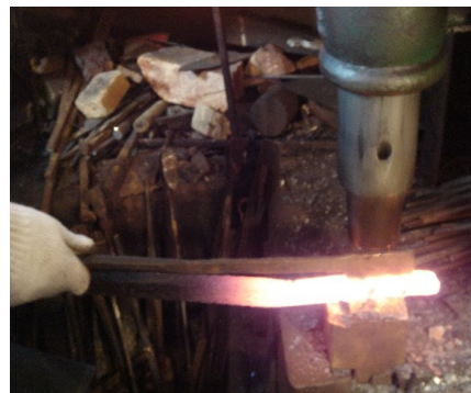
making the ditch of the Y section to put steel with chisel and belt hammer. It's so dangerous works!
