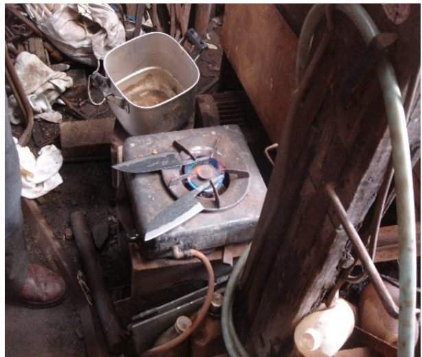
Burning core to fit handle
