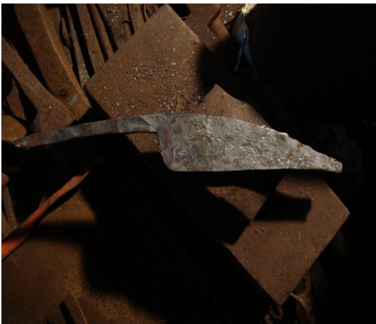
The part which is round of the back spreads at a stage postponing the part of the blade thinly and becomes straight.
