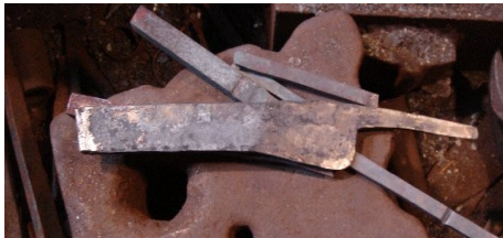
Heating again to stretch the another side.
