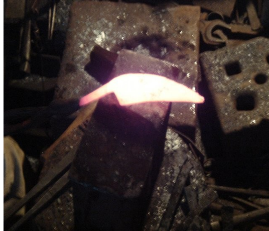
Next ,smiting a back like the form of the shrimp to be next. This is very important in a next process
