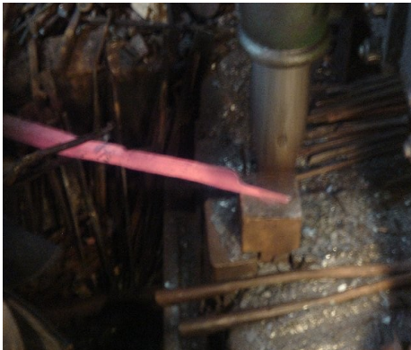
Stretching from center portion to make 2pcs length.
