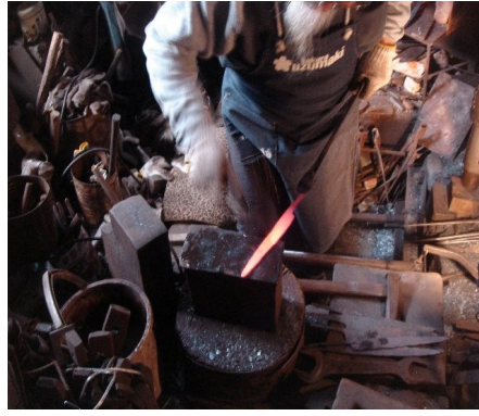
After heating ,smiting with watered hammer. Removing the garbage with phreatic explosion.
