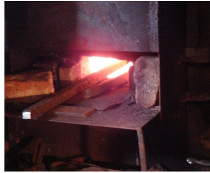
around 1,200 degrees and begin forging. The color is tinged with yellow
