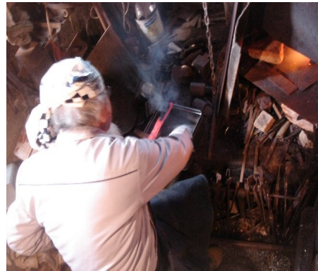
Boric acid ( H_3BO_3 ) helps hammer welding well.
